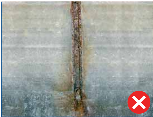
Rust formation when using non-corrosion-resistant materials subject to attack from acid or salt
